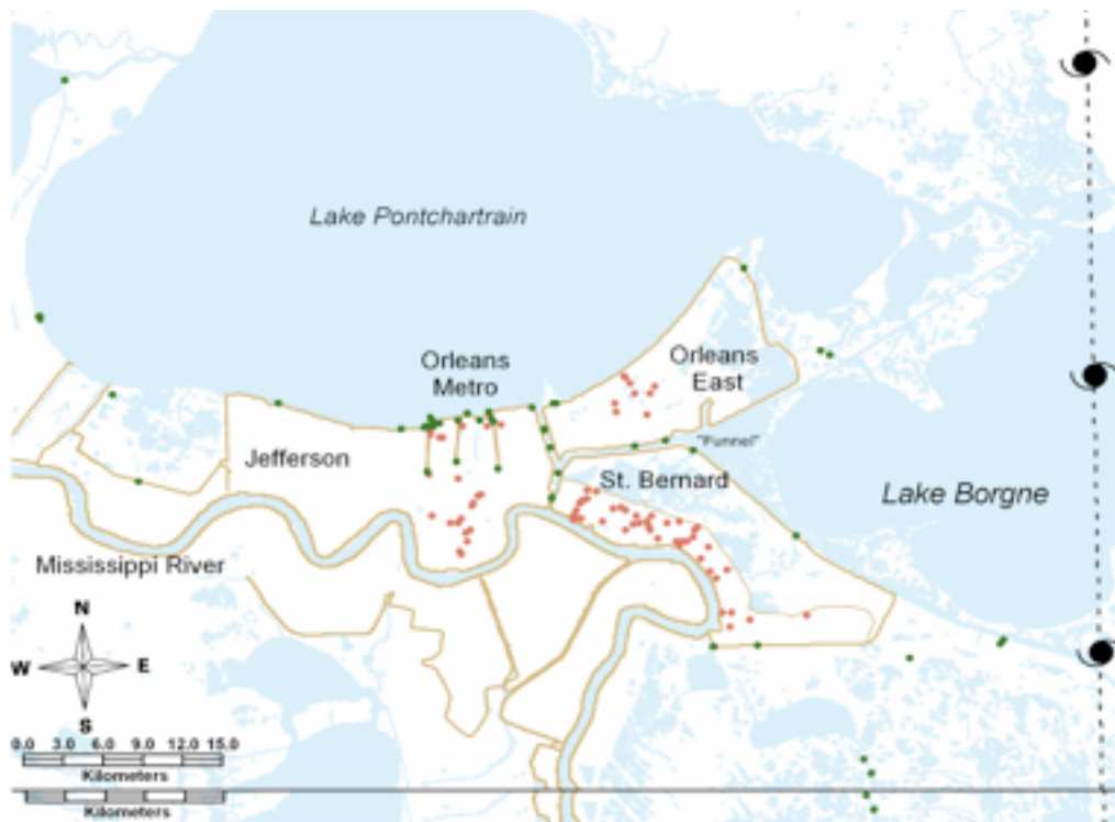
Figure 14. The “Funnel” Exposing New Orleans to Increased Storm Surge Damage
